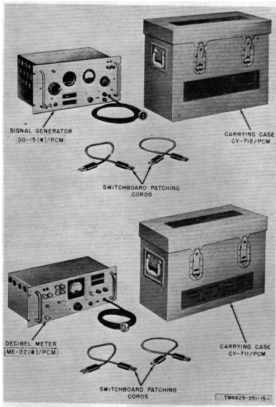
Figure 1-1. Test Set TS-140/PCM less running spares and technical manuals.
