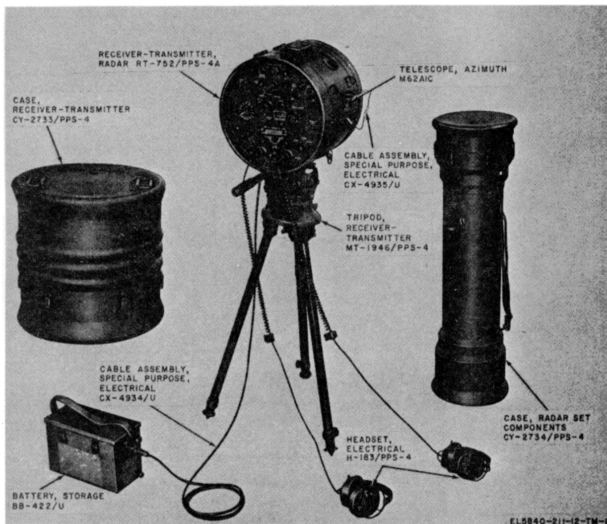
Figure 1-1. Radar Set AN/PPS-4A, components and auxiliary battery.
