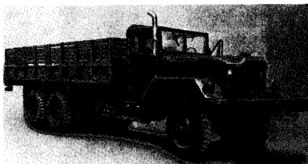
Figure 2-2. Truck, cargo, dropside, 5-ton, 6x6, M813A1.
